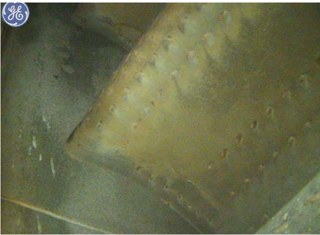
Discoloration on the HPT STG1 Blade LE
