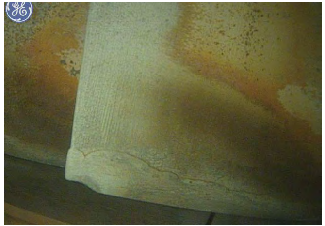
Discoloration on convex surface of STG1 blades and missing on the tip cap trailing edge corner. (only one blade)
