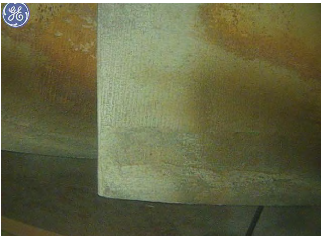
Discoloration on convex surface of STG1 blades and missing on the tip cap trailing edge corner. (only one blade)
