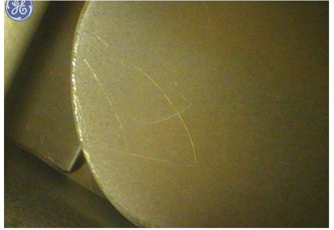
HPC STG13 Blade filed on L/E side
