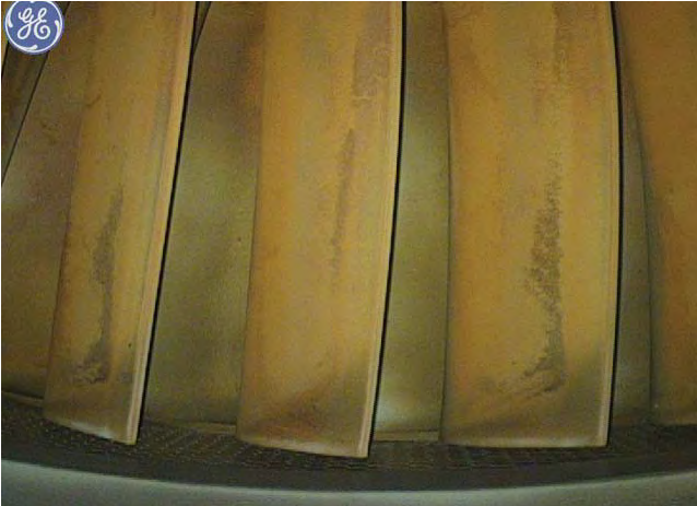
HPT STG2 Rotor Blades TE View
