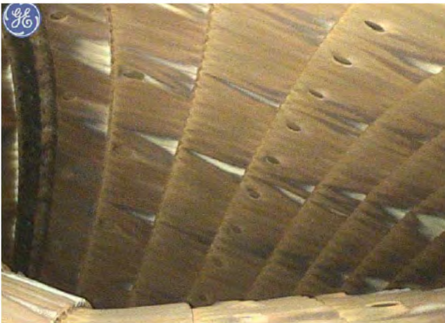
Combustor Outer Liner Condition observed some discoloration areas on the scoop louvers.
