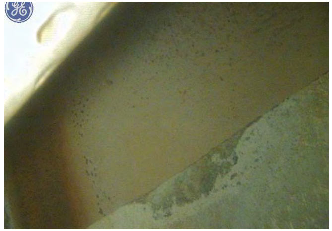
Eroded areas on the HPT STG1 Nozzle Vane Trailing edge side. Serviceable
