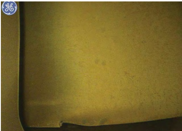
HPC STG12 Blade damage on Tip Cord area
