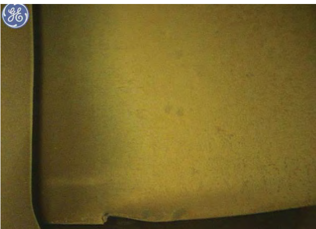
HPC STG12 Blade Nick on L/E Blade
